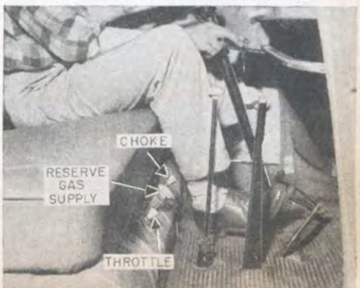
Line-up of controls and pedals. Stick shift is a standard H-pattern for four forward speeds. For reverse, you push stick down toward floor, then swing it to the left and down. Note wide and open glove compartment.
