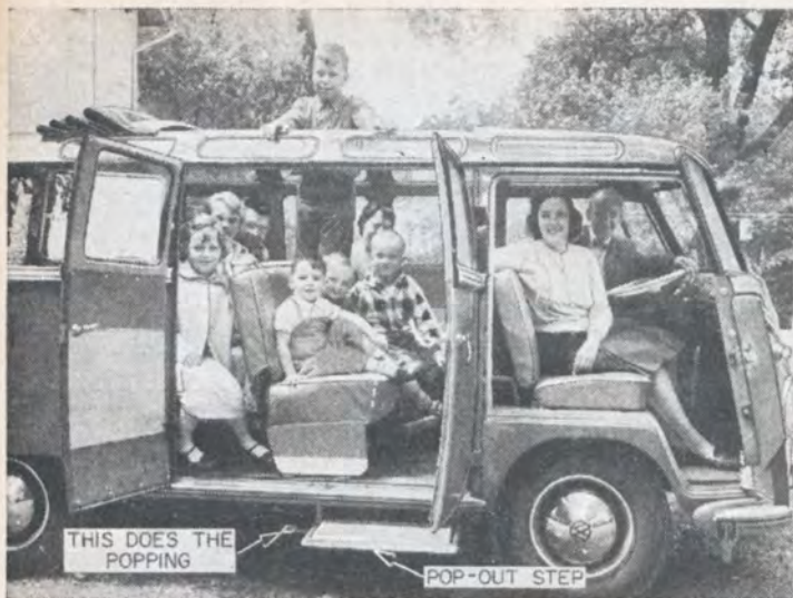
Just the thing for large families or Cub Scout packs. Entrance to the rear is aided (above) by spring-loaded step released by pedal. While bystanders will have no objection, getting in and out of the driver's seat (right) can be awkward for ladies, but getting into the front passenger's side is not too difficult (upper right) because of the fold-down step provided.
