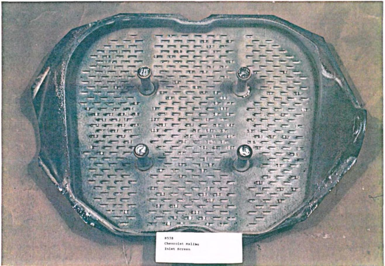
Photo 23. Converter #538 Inlet Screen
