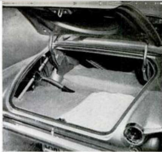
Roomy trunk results from locating tire under floor. This unfortunately makes filter pipe placement a problem
