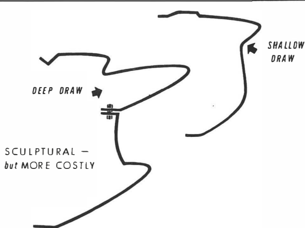
Fig. 14 - One piece and two piece panel sections
