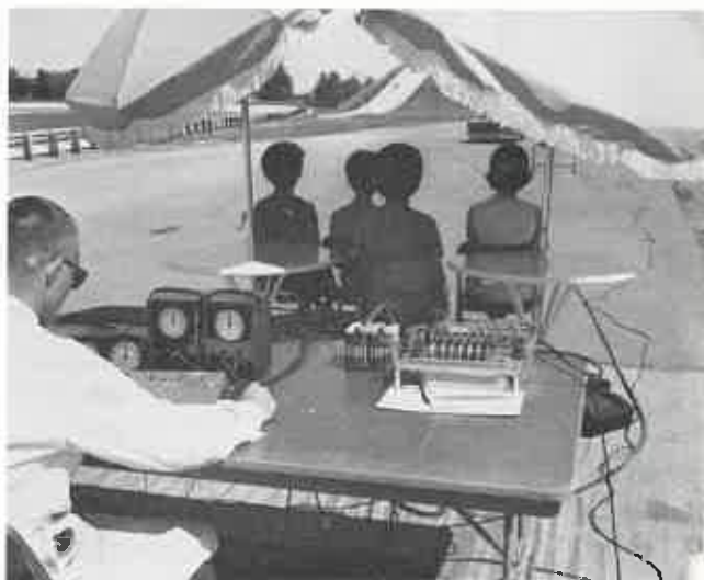
FIGURE II The experimental set-up showing the experimenter's station, subject's station, primary and secondary task lights.
