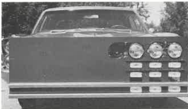
FIGURE 1 The secondary task light jig showing the turn signals and headlamps.
